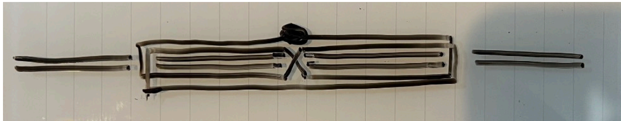
Diagram of hypothetical stitch path from the side, back of book 'up', knot at center. Copyright Jacqueline Chenault.
