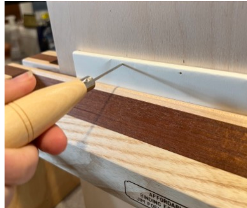
Piercing the book block with an awl to create the third stitching hole
