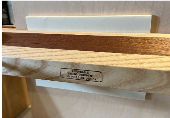
Book block with wrapped plain paper cover, secured against board in finishing press
