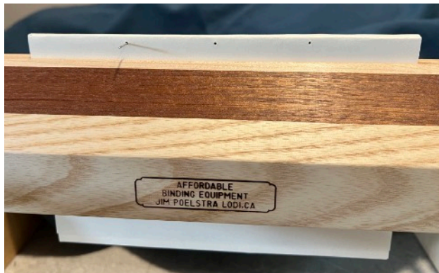
Board removed, checking and slightly enlarging holes with a needle
